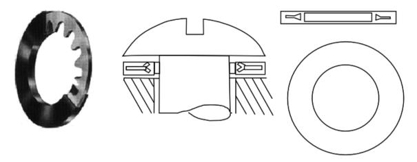
The shakeproof washer is well known for its ability to resist vibration, the effect of tightening the bolt or nut causing the metal serrations to pierce the rubber, bite into the relative metal surface and thus providing the necessary locking action. The covering or rubber reduces the risk of corrosion that would occur with a normal lockwasher by enveloping the scores in the protective treatment on the metal face to give effective protection against moisture and oxidation.
